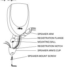
Remove base from Satellite by unscrewing the Adjustment Screw. See the Owner's Guide for your Modulus Speakers for more details. Set a Satellite into one of the Speaker Arms and align it so that the Registration Flange fits into the Registration Notch. Using the larger Allen Wrench, fasten the Speaker-Mount Screw into the bottom of the Satellite's mounting ball and tighten. Repeat Step Seven for other Satellite.
