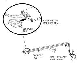
Slide one Support Pad into the open end of the Right-Side Speaker Arm, as shown in the drawing. Repeat for the Left-Side Speaker Arm. These Support Pads help distribute the weight of the Modulus TV Bracket across the top of your television. NOTE: There are two types of Support Pads. Use only the type that provides the best support of the bracket for the contour of your television. See Step 5.
