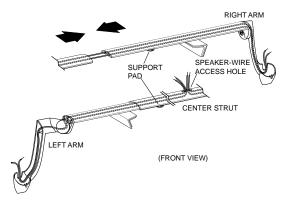
Slide the Left- and Right-Side-Arm Assemblies into the ends of the Center Strut with the Speaker-Wire Access Hole toward the rear. The Modulus TV Bracket is designed to hide the Speaker Wires by running them through the Center Strut and out the Speaker-Wire Access Hole. To help support the wire, attach the two Wire-Guide Tabs to the Center Strut by clipping them into place. Run the open end of the excess Speaker Wire from each Arm Assembly out through the Speaker-Wire Access Hole.
