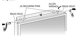
Due to the Modulus TV Bracket's length, two people should be used to mount it on the TV. Have one person press the two ends toward each other so that the L-Shaped Clamps snugly hold the sides of the TV between them. Have the other person use the smaller Allen Wrench to tighten the four Securing Pins on the rear of the Center Strut.
